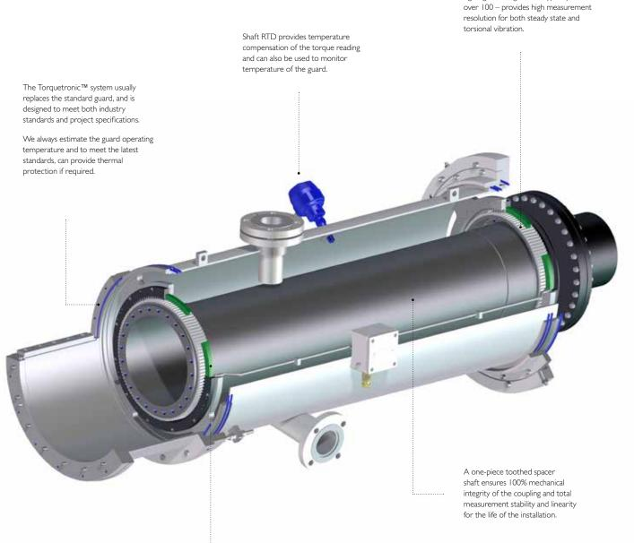
There are no rotating electronics fitted to the torsion shaft. Signals are generated in fully encapsulated stationary coils that are rated for operation at up to 150°C and a life in excess of twenty years.
